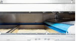
warm air through the grater. The direction in which the air is blown changes frequently to ensure that the cheese is equally dried. The drying takes about 90 minutes. With this drying tunnel, we have three times more capacity than before. If one module fails, we still have more than 90% capacity available. This is ideal."
