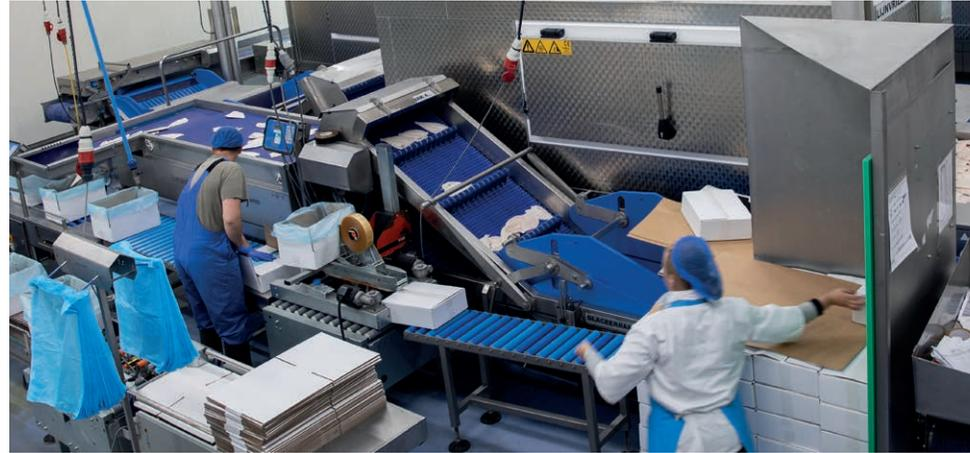
After treatment in the air blast freezer the fish is so hard that it no longer needs to be laid on the belt spread out, but can be laid one on top of the other. “The plant involved in the post-freezing process gives the fish a lovely ice layer. Seeing the product after this phase often leaves customers speechless. That's because the frozen product looks even better than the fresh product,” he says.
